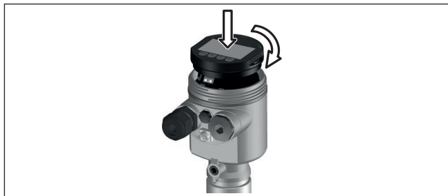
Fig. 23: Installing the display and adjustment module in the electronics compartment of the single chamber housing
