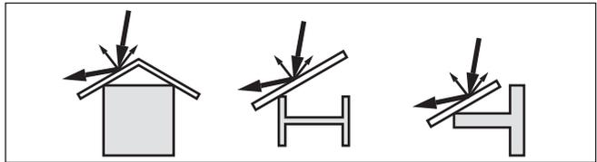
Fig. 11: Cover flat, large-area profiles with deflectors
