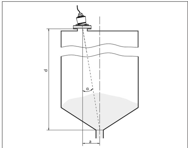
Fig. 14: Proposal for installation after orientation VEGAPULS C 11
