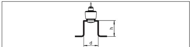
Fig. 10: Socket mounting with deviating socket dimensions
