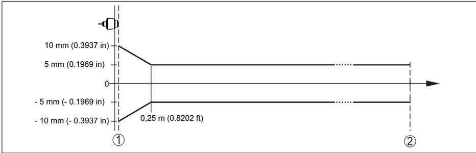
Fig. 26: Deviation under reference conditions<sup>7)</sup>
