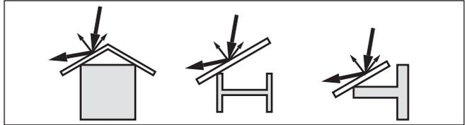
Fig. 10: Cover flat, large-area profiles with deflectors
