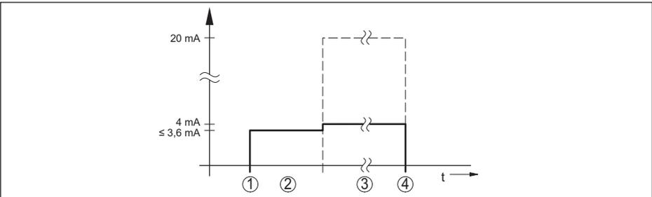
Fig. 25: Run-up time and measured value output
