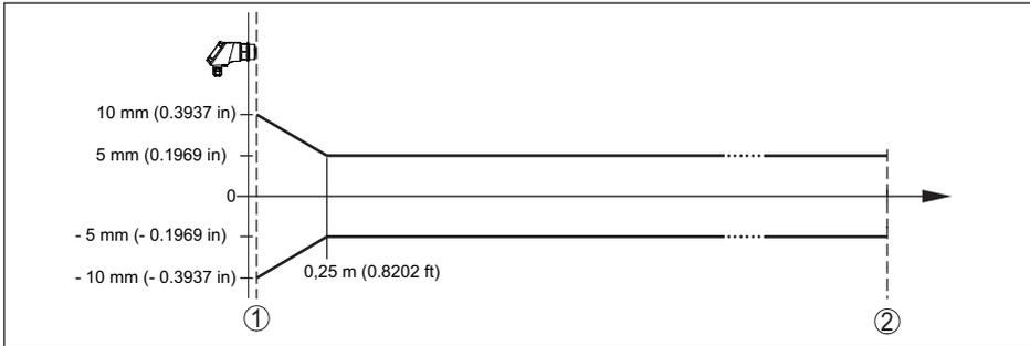
Fig. 26: Deviation under reference conditions<sup>8)</sup>
