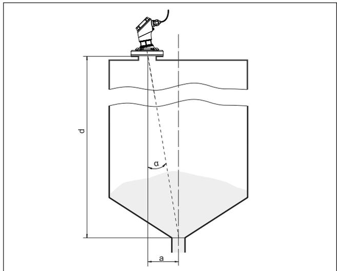
Fig. 13: Proposal for installation after orientation VEGAPULS 11
