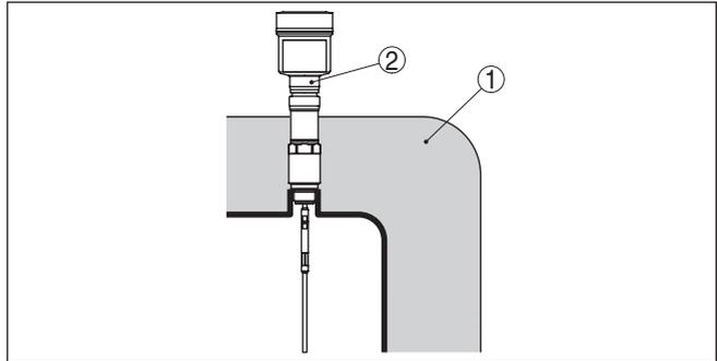
Fig. 10: Mounting the instrument on insulated vessels.
