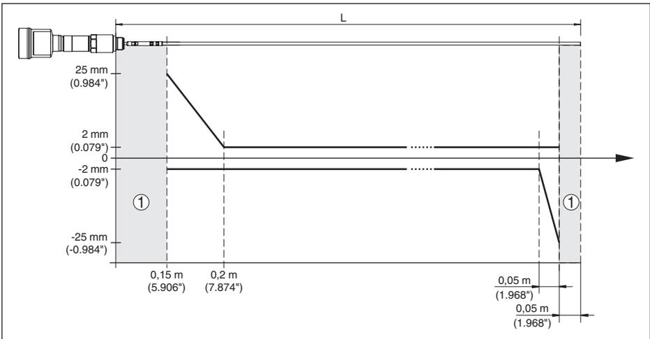
Fig. 41: Deviation VEGAFLEX 86 in rod version in oil
