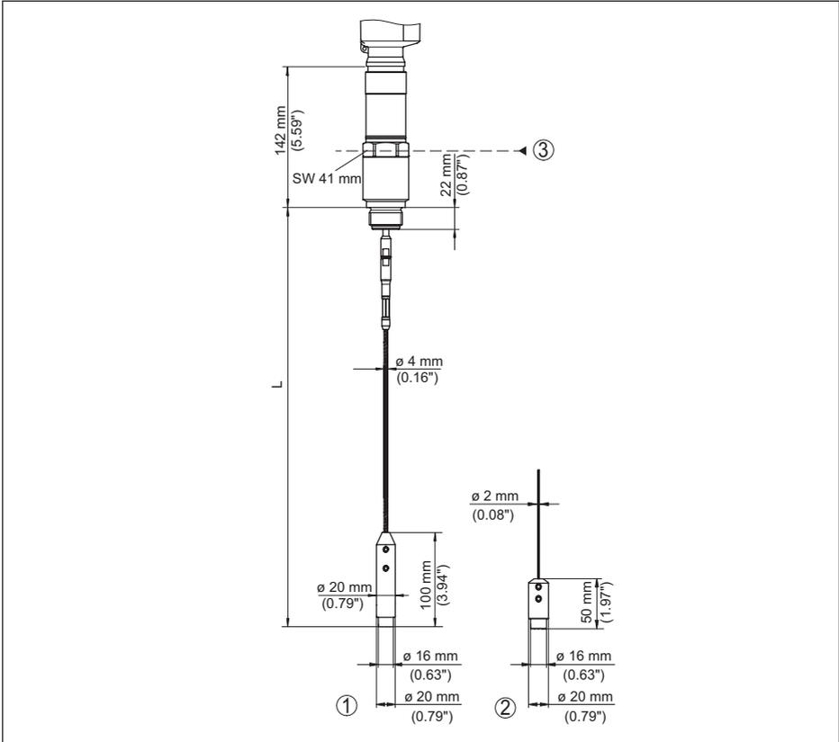
Fig. 51: VEGAFLEX 86, threaded version with gravity weight (all gravity weights with thread M8 for eye-bolt)
