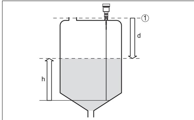
Fig. 1: Level measurement
