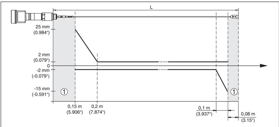
Fig. 43: Deviation VEGAFLEX 86 in cable version (ø 2 mm/0.079 in), in medium oil
