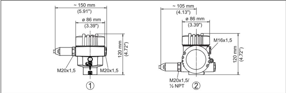
Fig. 48: Housing versions with protection rating IP66/IP68 (1 bar), (with integrated display and adjustment module the housing is 18 mm/0.71 in higher)
