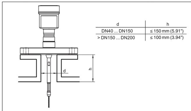
Fig. 5: Mounting socket
