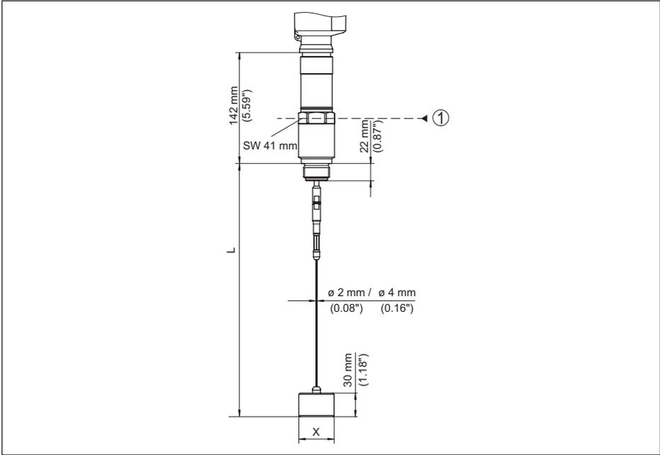
Fig. 52: VEGAFLEX 86, threaded version with centering weight
