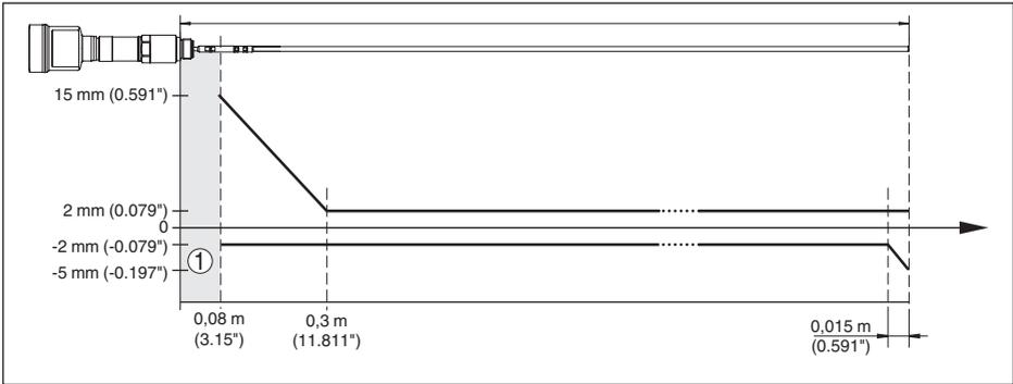
Fig. 40: Deviation VEGAFLEX 86 in rod version in water
