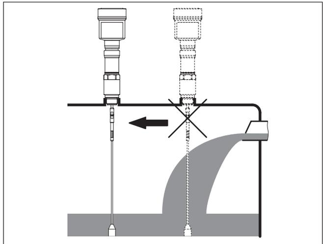
Fig. 7: Mounting of the sensor with inflowing medium
