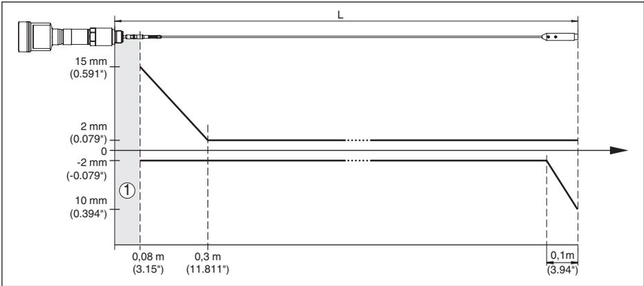
Fig. 42: Deviation VEGAFLEX 86 in cable version in water
