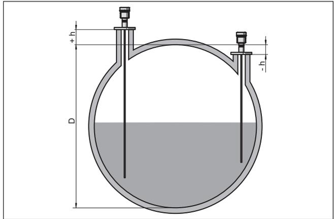
Fig. 28: Vessel height and socket correction value
