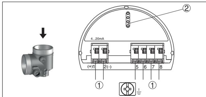
Fig. 15: Electronics compartment - double chamber housing
