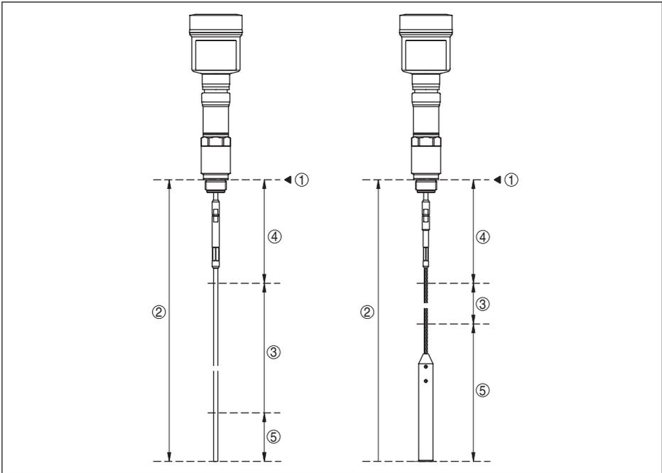
Fig. 39: Measuring ranges - VEGAFLEX 86
