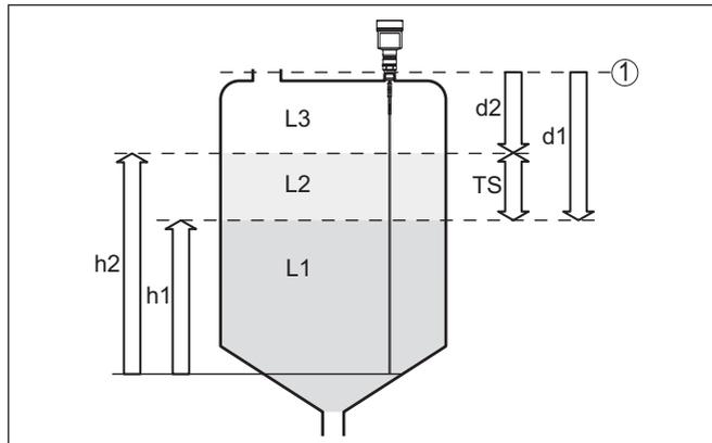
Fig. 2: Interface measurement
