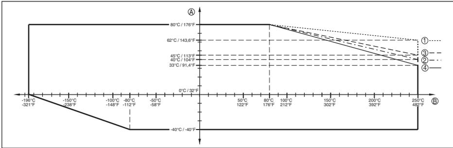
Fig. 45: Ambient temperature - process temperature, standard version
